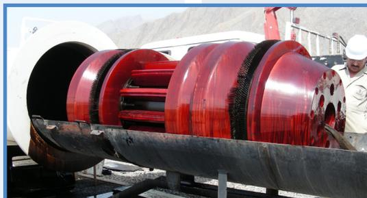
A 42 IN. CUP PIG WITH CHECK VALVE USED FOR A CRUDE PIPELINE PROJECT IN OMAN.
