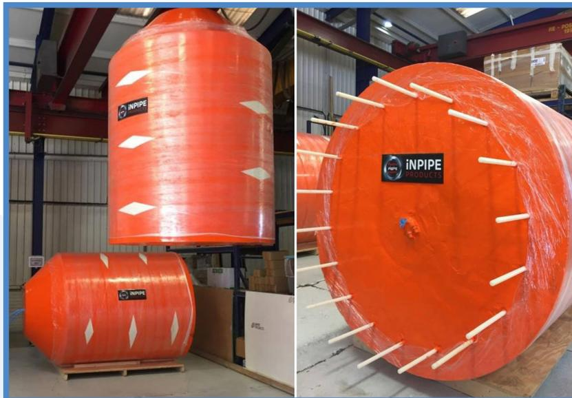
LEFT: TWO LRSD 68 IN. CRISS-CROSS FOAM PIGS COMPLETE WITH NYLON PULLING ROPE. RIGHT: ONE 1600 MM OD FULLY COATED PIG COMPLETE WITH STUDDING FOR FITTING A GAUGE PLATE.
